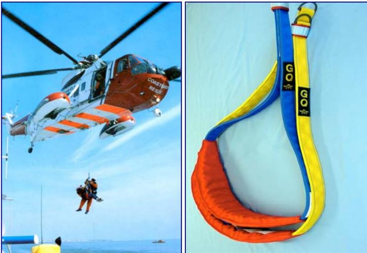
The Hypothermic Lift Strop when used in conjunction with a standard rescue strop, allows survivors suffering from hypothermia to be lifted horizontally into the aircraft thus minimising the risk of a post rescue loss of blood pressure.
