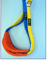
The Hypothermic Lift Strop when used in conjunction with a standard rescue strop, allows survivors suffering from hypothermia to be lifted horizontally into the aircraft thus minimising the risk of a post rescue loss of blood pressure.
